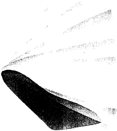
FIGURE 5.28 Calculated 3-dimensional shock-wave shape on a shuttle-like configuration. (From Weilmuenster, Ref. 68.)
